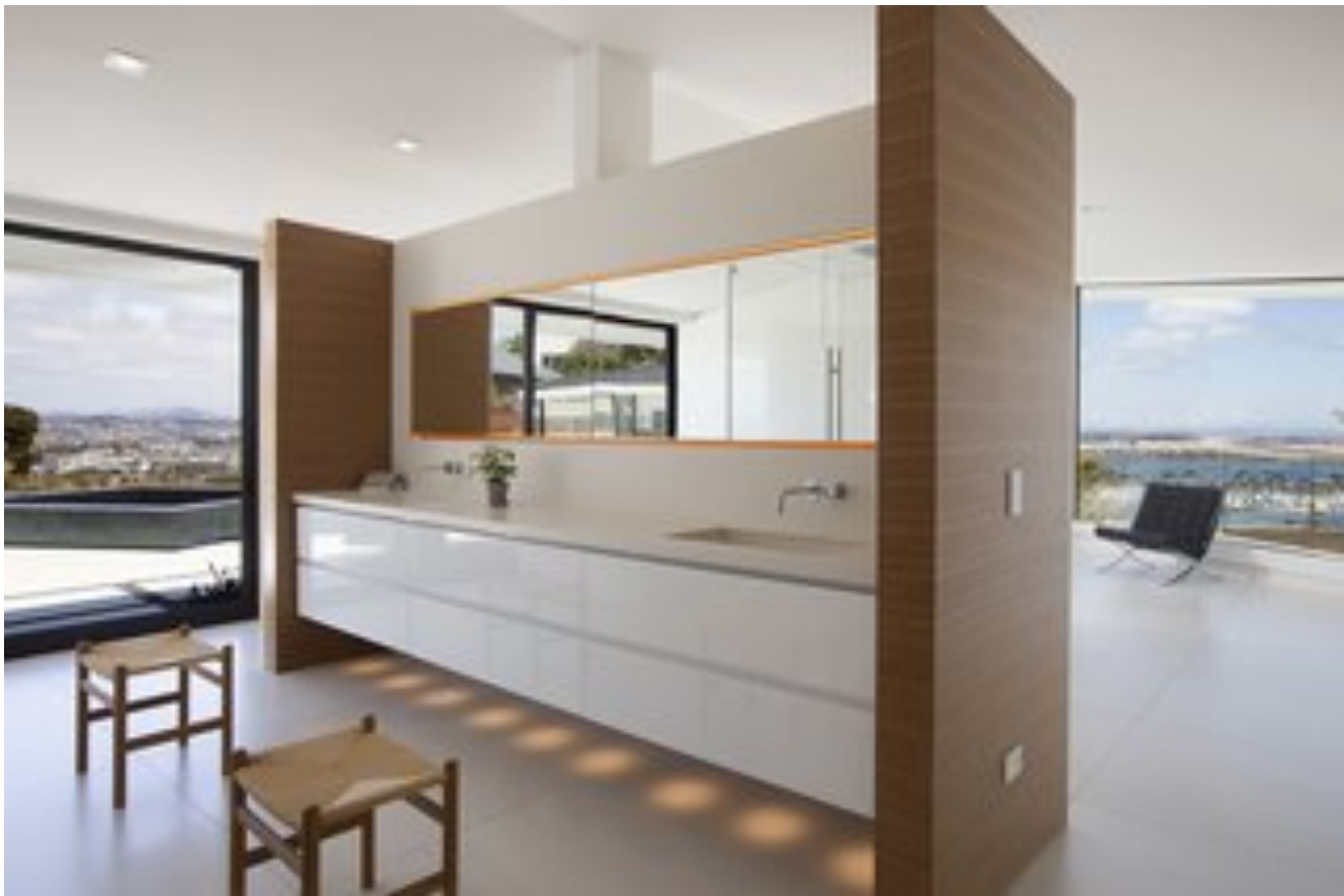
Low-emission, 45-inch by 60-inch Italian ceramic floor tiles were used throughout.
